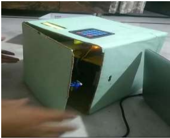
Fig a): When we enter password correctly through keypad. Servo motor rotates 180 degree and the door opens. When we press “#” the door closes.
