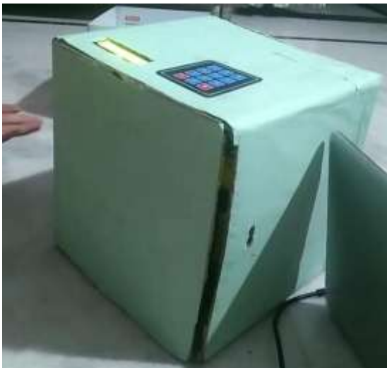
Fig b): When we enter incorrect through keypad. The door remains closed and buzzer beeps
